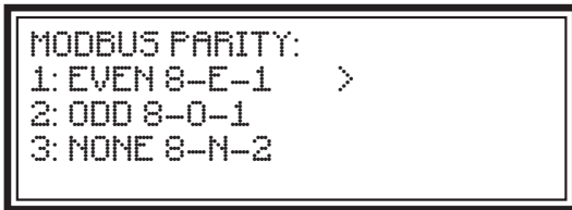
Modbus Parity Setting
