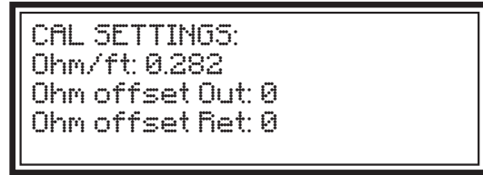
Current Calibration Settings Screen
