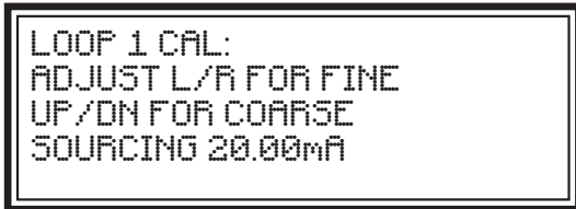
Loop 1 - 20mA Calibration Screen
