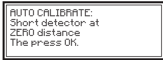
Zero Calibration Start Screen
