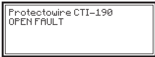
Open Fault Display
