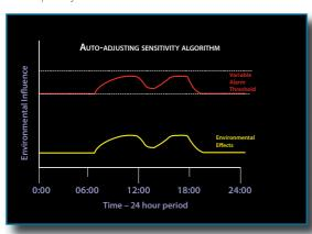
Automatic drift compensation prevents the long-term build up of dust or dirt on the optical surfaces from making the detector more sensitive; the design of the enclosure also ensures that settling dust attenuates the optical path as little as possible. The sensitivity of the detector can be set to one of four levels between 25% and 50% obscuration, providing application flexibility to suit the environment in which the detector will be installed.
