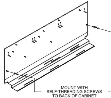
The BB-XP cabinet has a built-in chassis that will accommodate one or two XP10-M modules.
