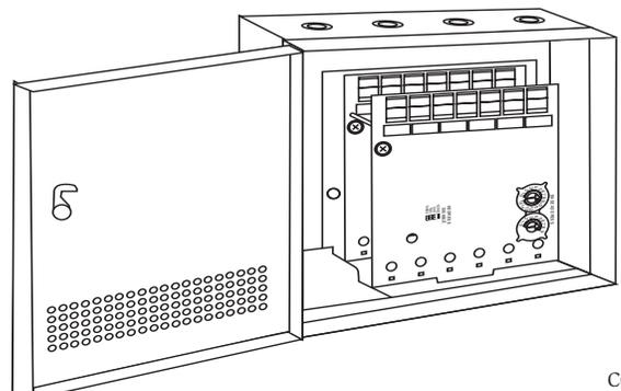
The front XP10-M module positions of each chassis are offset below the rear XP10-M module positions so that all of the status indicators are visible.
