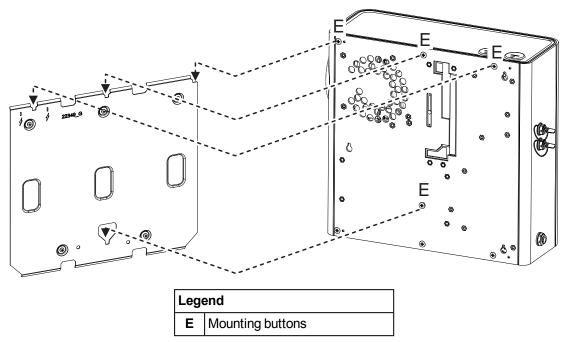
Figure 4-6: Mounting the detector
