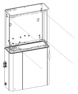
Figure A-34: Tighten Mounting Screws
