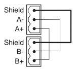
Figure 4-16: Closed loop for standalone detectors with VESDAnet capability
