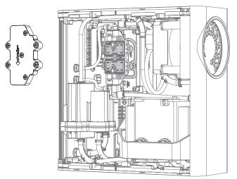
Figure 7-6: Lift the filter out from the detector
