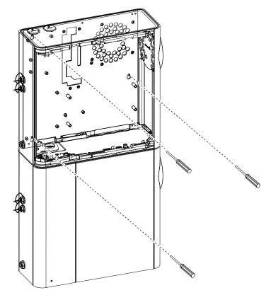
Figure A-14: Tighten Mounting Screws
