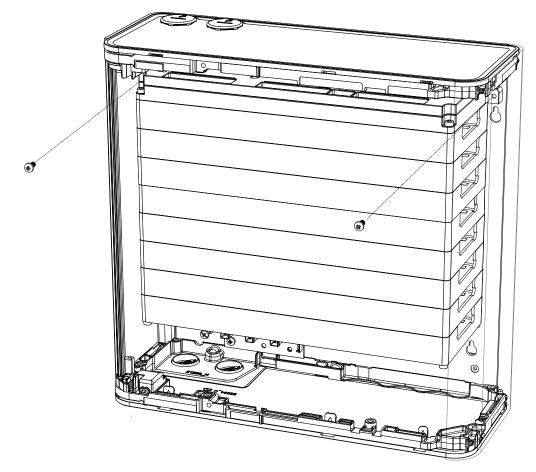
Figure A-39: Secure Trays to the enclosure
