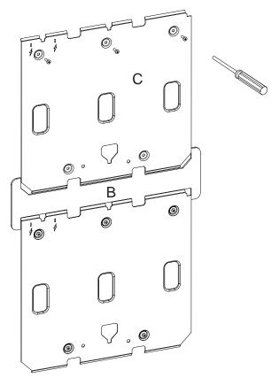
Figure A-27: Position and secure the Local Relay StaX Mounting Bracket
