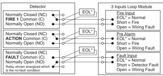
Figure 4-18: Input/Output Loop Module with EOL
