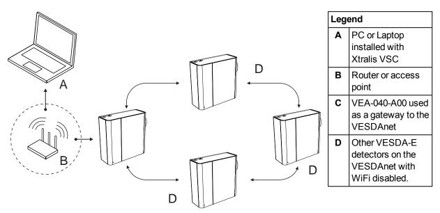
Figure 5-11: Connection to a detector via another detector on VESDAnet using a WiFi connection
