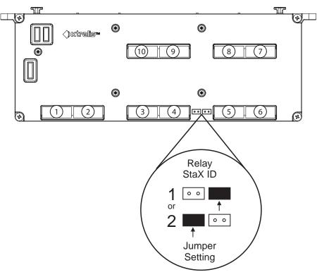
Figure A-41: Relay Module Configuration Jumpers
