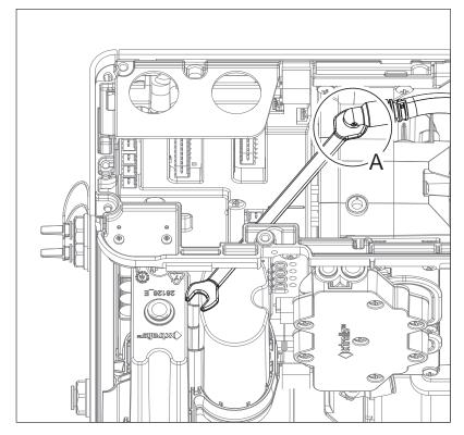
Figure 7-30: Disconnect pipe
