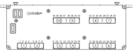
Figure A-35: Local Relay StaX Distribution Board
