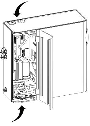
Figure 4-13: Cabling Inlets
