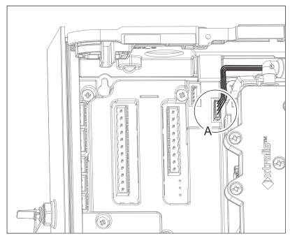
Figure 7-29: Remove the smoke sensor cable
