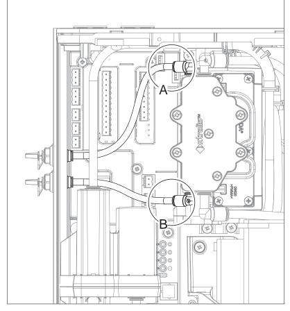
Figure 7-26: Smoke Test Port Pipes
