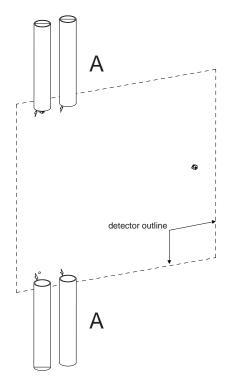
Figure 4-10: Cut the electrical conduit
