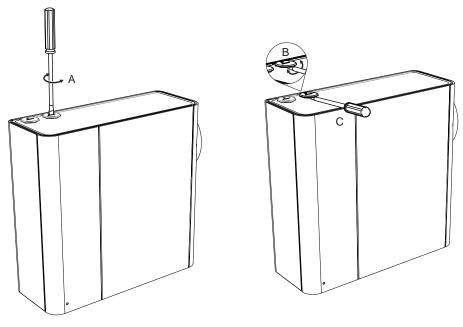
Figure 4-2: Remove Cable and Conduit Inlet Plugs
