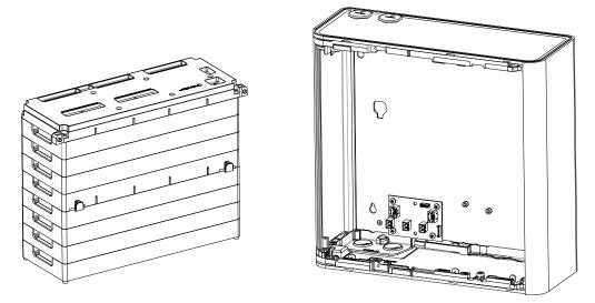
Figure A-38: Insert Trays into the enclosure
