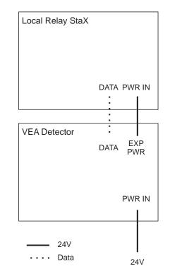
Figure 4-20: Single VEA detector and Expansion StaX
