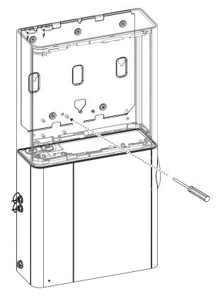
Figure A-9: Secure the Expansion StaX to its mounting bracket
