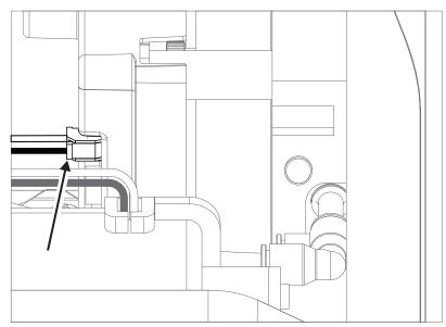
Figure 7-20: Disconnect power cable
