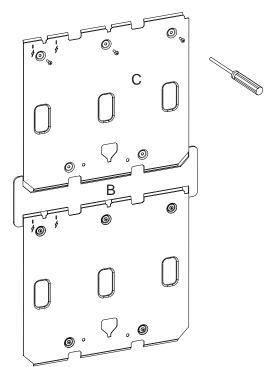
Figure A-7: Position and secure the Expansion Stax Mounting Bracket
