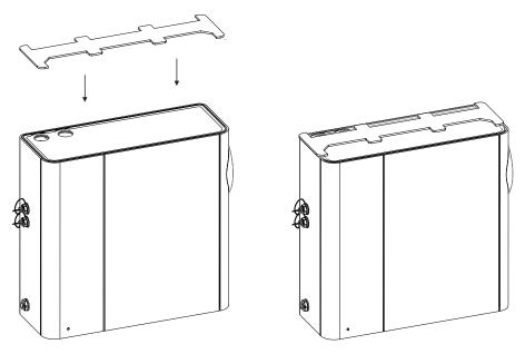
Figure A-30: Place the Mounting Bracket spacer on top of the detector
