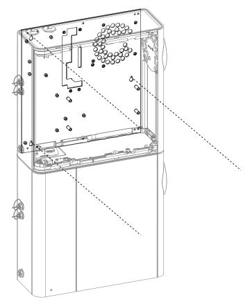
Figure A-11: Mark pilot hole positions on the mounting surface
