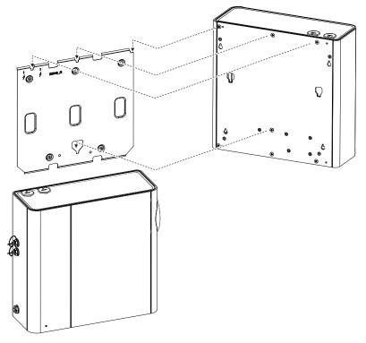
Figure A-8: Fit the Expansion StaX to its mounting bracket
