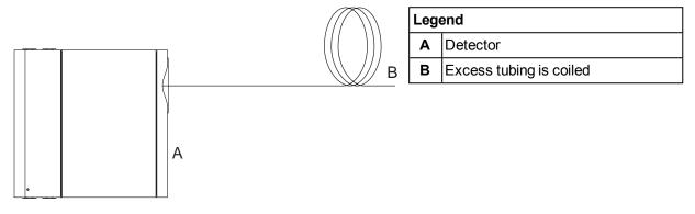
Figure 3-1: Configuration with equal length tubes
