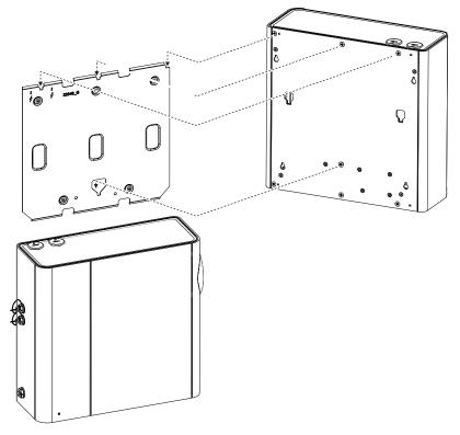
Figure A-28: Fit the Local Relay StaX to its mounting bracket
