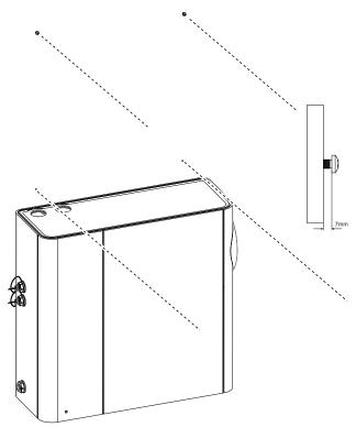
Figure A-32: Insert mounting screws
