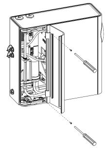
Figure 7-3: Fascia removal - remove screws
