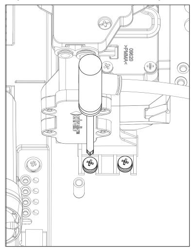
Figure 7-32: Remove Smoke Sensor Module retaining screws
