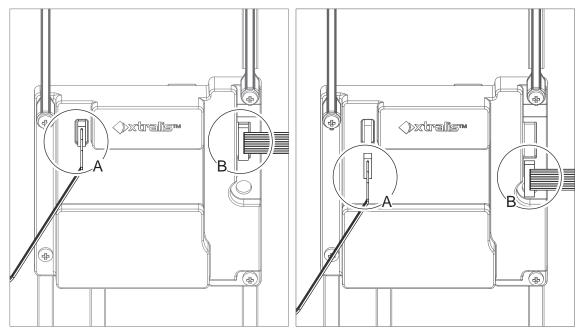
Figure 7-4: Disconnect the LCD and LED looms
