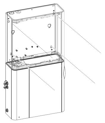
Figure A-31: Position mounting template
