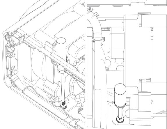
Figure 7-22: Remove rotary valve retaining screws
