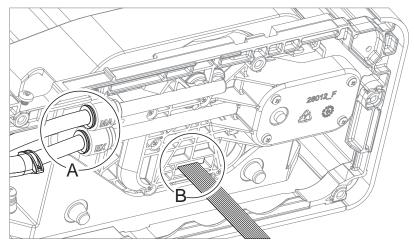
Figure 7-10: Remove pipes and cable
