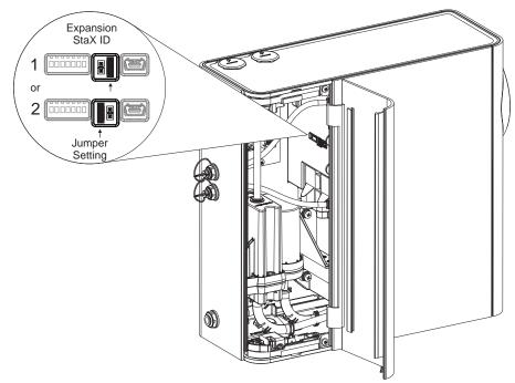
Figure A-18: Expansion StaX address configuration
