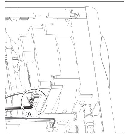
Figure 7-25: Disconnect data loom
