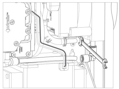
Figure 7-18: Disconnect pipe
