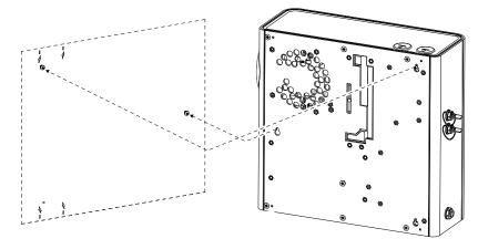
Figure 4-11: Mount the detector
