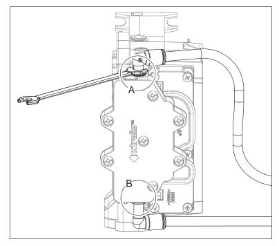
Figure 7-33: Remove Smoke Sensor Module
