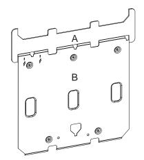
Figure A-6: Position the Mounting Bracket Spacer above or below the detector mounting bracket
