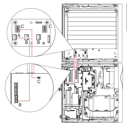
Figure A-36: Power and Data Wiring
