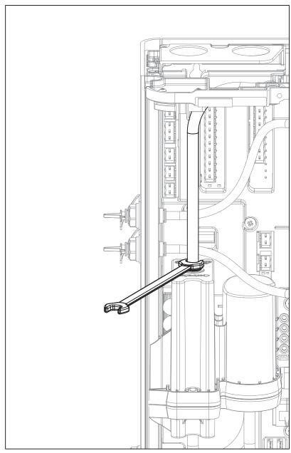
Figure 7-28: Remove the pipe
