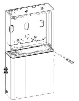
Figure A-29: Secure the Local Relay StaX to its mounting bracket
