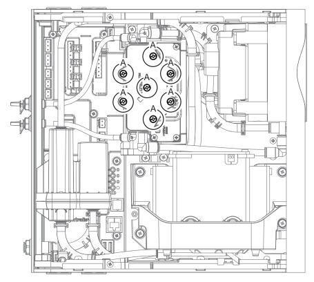
Figure 7-5: Remove filter retaining screws
