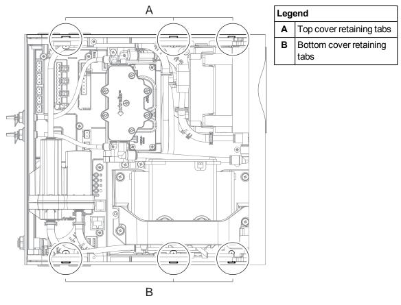
Figure 7-9: Tabs used to remove top and bottom cover
