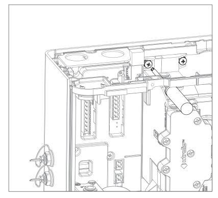
Figure 7-31: Remove Smoke Sensor Module retaining screws
