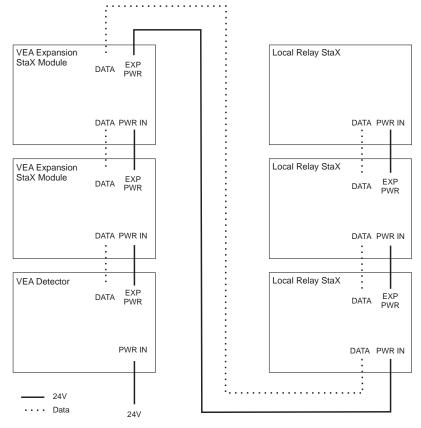
Figure 4-22: Multiple Module System
