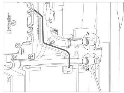
Figure 7-17: Disconnect pipes
