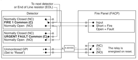
Figure 4-17: Typical wiring to a fire panel with EOL
