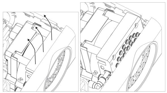
Figure 7-23: Remove rotary valve
