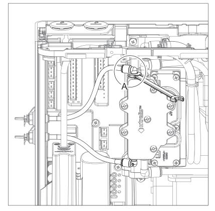
Figure 7-27: Disconnect Smoke Test Port Pipes
