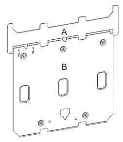
Figure A-26: Position the Mounting Bracket Spacer above or below the detector mounting bracket
