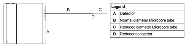
Figure 3-2: Configuration with mixed diameter tubes
