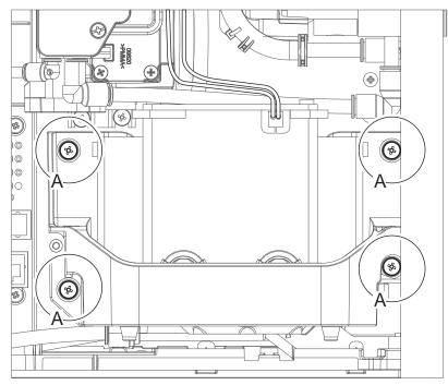
Figure 7-14: Remove pump retaining screws
